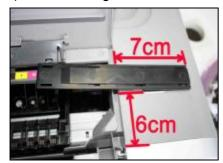
Attache the support arm on the proper position as the picture shown above.
